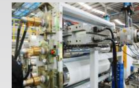
DIE HEAD ■ PE-APCP Extruding production line:T mold.
